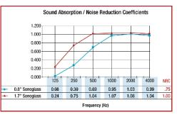
Noise Reduction Coefficient ASTM C423:
